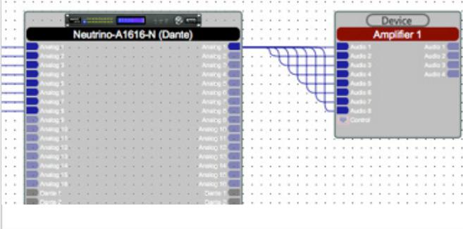
b) Click and drag each wire using the red nodes to move and stack the wires.
