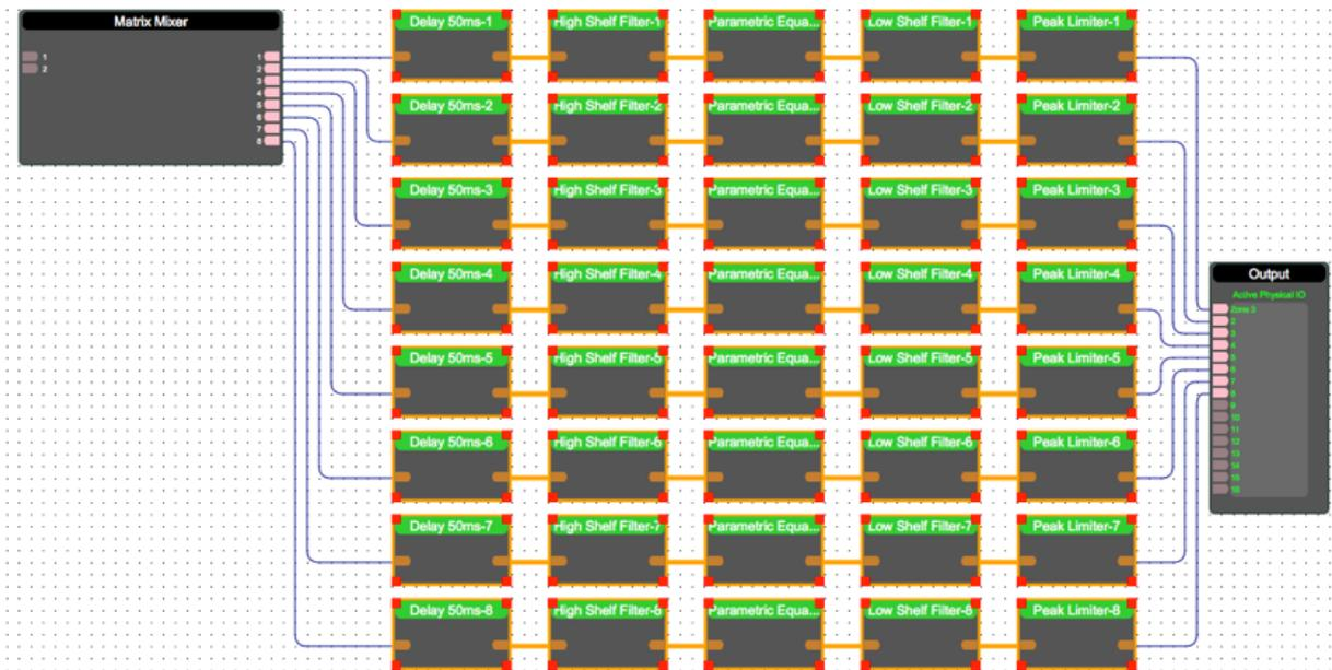
Adjust the module size by clicking and dragging a red corner node or adjusting the width and height in the Object Property menu.
