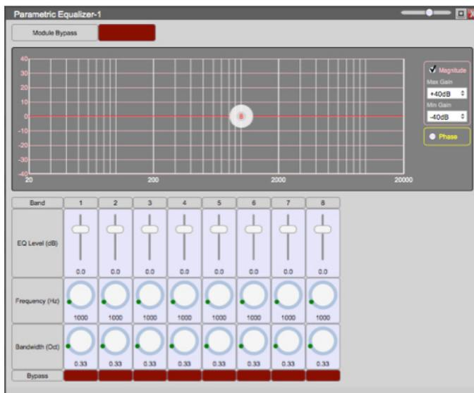
When multiple DSP Modules will need the same or similar settings, the first module can be set up, then copied and pasted.
