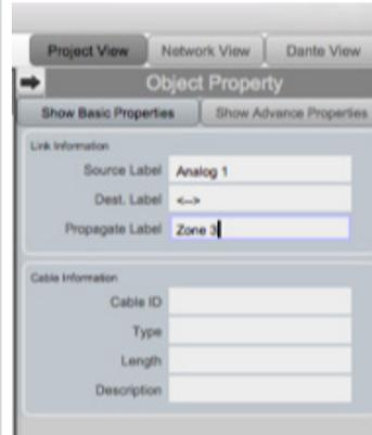
c) The input and output nodes will be renamed with the propagate label.
