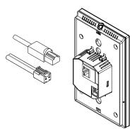
If you are using an external power adapter/source, connect the 2 Pin connector of the adapter/source to XTouch50 power jack.
