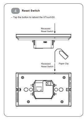
The XTouch50 has been designed to provide years of trouble free operation when wired and installed properly.
