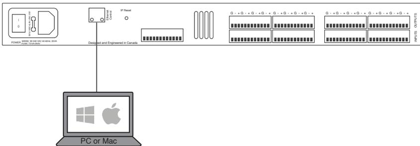
All wired connections use a standard RJ45 Cat 5/6 (Ethernet) connection.
