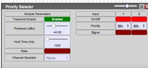
Multiple channel input, single output. Output is the input On channel with highest Priority (First-Tenth) channel above the Threshold (-60dB to 0dB) value when Threshold Enable is activated. Includes output Mute, Hold Time (10ms to 30s), signal (above threshold) and Channel Selection indicators
