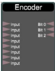
Convert eight GPIO inputs to three binary inputs. The module shows encoded Channels.
