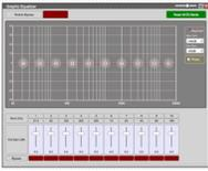
Increase/decrease the EQ Level (-30dB to +15dB, 0.1dB steps) within 10, 15 or 31 bands across the frequency range. Set the number of bands in Component Properties. Bypass feature included for each band
