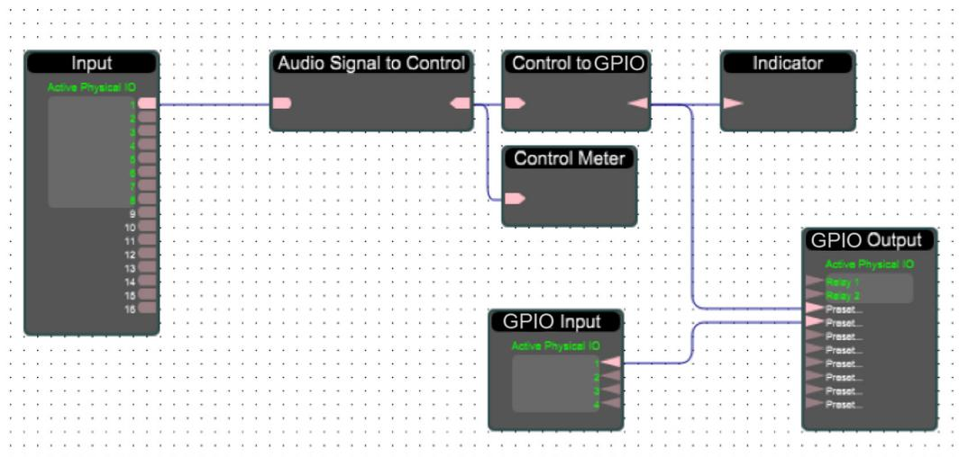
In the above example, the audio signal is converted to Control, and the Control is then converted to GPIO.
