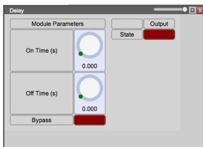
When the input is GPIO high for at least the On Time (0 to 60s, 1ms steps) the output will be GPIO high for the on time and GPIO low for the Off Time (0 to 60s, 1ms steps). Bypass and output State indicator features present.
