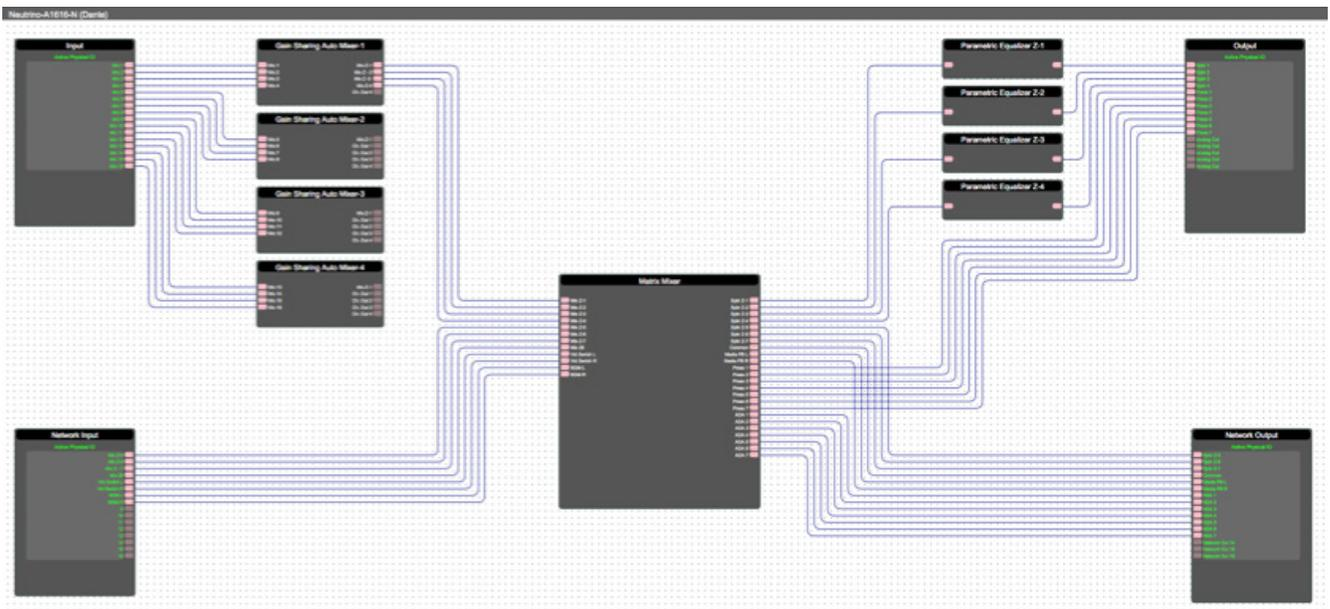
Example of the internal configuration inside the second Neutrino A1616-N DSP or "Unit 2":
