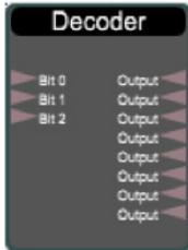
Convert three binary inputs to eight GPIO inputs. The module shows decoded Channels.
