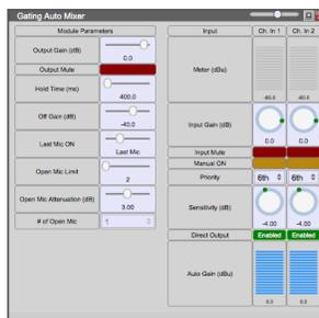
Typically used in a conference setting where multiple MICs are in use but only one (or a few) should be on at any time. This module turns on MICs based on their input signal as compared to the level of the other MICs. Once a channel is activated it typically stays on until another signal is larger. Includes: Mute and Gain (-100 to 16 dB, 0.01dB steps), RMS Meter (-80 to 40 dB, 0.1 dB steps) and Auto Gain meter (-100 to 0 dB, 0.1 dB steps)
