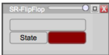
For each trigger (low-to-high signal) at the Trigger pin, Output Q will switch GPIO values. The module displays the current State of the Q pin. Output /Q is always the opposite of Output Q. While the Set pin is GPIO high Output Q will be GPIO high and While the Reset I/O is GPIO high Output Q will be GPIO low.
