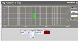
Attenuates frequencies below target Frequency (20Hz to 20kHz, 1 Hz steps and with filter Type (Butterworth, Linkwitz-Riley and Bessel) and Slope (6 to 48dB/oct, 6dB/oct steps.) Bypass feature included
