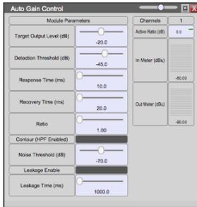
Keeps the volume at a set level. When the input is below a threshold, it will amplify to bring the level up to the Target Output Level, and when over will reduce the gain to bring it back below the Target output Level.
