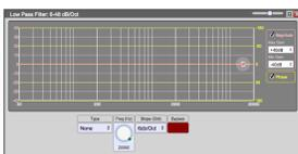
Attenuates frequencies above target Frequency (20Hz to 20kHz, 1 Hz steps) with filter Type (Butterworth, Linkwitz-Riley and Bessel) and Slope (6 to 48dB/oct, 6dB/oct steps). Bypass feature included
