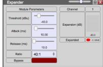
Reduces the signal level below the Threshold (-60 to 20dB, 0.1 dB steps) value by the Ratio (1:1, 40:1, 1:1 steps) set. Attack (0.1 to 100ms, 0.01ms steps) adjusts the time to reduce the signal once the signal has dropped below the threshold. Once the signal has risen above the threshold the Release (0ms to 10s, 1ms) time is the time to stop compressing the signal. Bypass feature and RMS meter included
