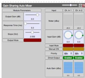
Allows the automatic mixing of input channels to one output channel based on input signal levels. The louder the particular input channel, the louder it will be at the output channel. Each input includes Mute, Gain (-100 to 16 dB, 0.01dB steps), RMS Meter (-80 to 40 dB, 0.1 dB steps) and Auto Gain meter (-100 to 0 dB, 0.1 dB steps) (Shows calculated gain for each channel)
