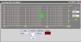
Attenuates frequencies above target Frequency (20Hz to 20kHz, 1 Hz steps) with filter Type (Butterworth, Linkwitz-Riley and Bessel) and Slope (6 to 24dB/oct, 6dB/oct steps). Bypass feature included
