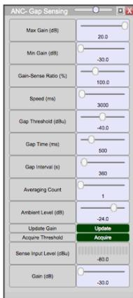
Used for speech & paging applications. The output level is adjusted automatically in response to variations in the ambient noise level. The ambient noise is measured in the output gaps, when no signal to the outputs is present, or drops to below a pre-defined threshold
