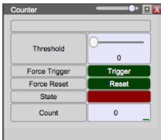
Each trigger (low-to-high signal) at the Trigger I/O adds one to the Count (0 to 99999999); at Threshold (0 to 99999999) the output state becomes high. State indicates the current output condition. Use Force Trigger to add one to the count total. Force Reset and a trigger (low-to-high signal) at the Reset I/O will reset the Count value to zero.
