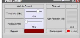
Reduces the signal level above the Threshold (-60 to 20dB, 0.5 dB steps) value by 40:1. Bypass feature and RMS meter included
