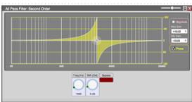
Unity gain filter, 180 deg. phase shift at target Frequency (20Hz-20kHz, 1 Hz steps) with roll off controlled by the Bandwidth (0.01to 4.00oct, 0.01 steps). Bypass feature included
