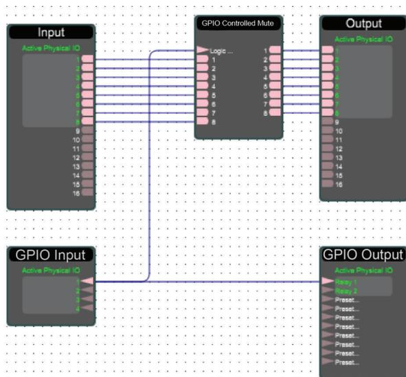
In the example above, notice that the input signal and Relay 1 is being routed to the GPIO Controlled Mute. One practical use for this configuration is having an external LED light up when the emergency mute button is active.
