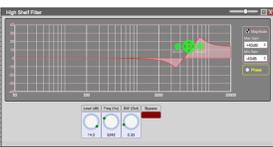
Increase/decrease frequencies above target Frequency (20Hz to 20kHz, 1 Hz steps) by the EQ Level (-30 to +15 dB, 0.1dB steps). Roll off controlled by the Bandwidth (0.01 to 4.00oct, 0.01 steps) setting. Bypass feature included
