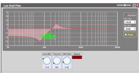
Increase/decrease frequencies below target Frequency (20Hz to 20kHz, 1 Hz steps) by the EQ Level (-30 to +15 dB, 0.1dB steps). Roll off controlled by the Bandwidth (0.01 to 4.00oct, 0.01 steps) setting. Bypass feature included
