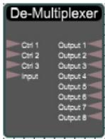
Route the input to one of the eight outputs using the three Ctrl (Control) I/O's. The module shows the channel selected.
