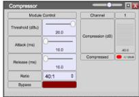
Reduces the signal level above the Threshold (-60 to 20dB, 0.5 dB steps) value by the Ratio (1:1, 40:1, 1:1 steps) set. Attack (0.1 to 2000ms, 0.1ms steps) adjusts the time to reduce the signal once the signal has been exceeded. Bypass feature and RMS meter included
