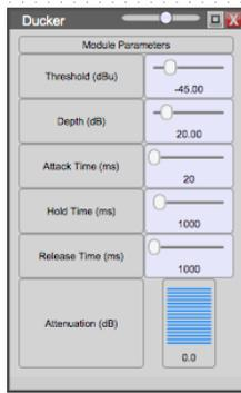
Attenuates channel 1 input by the Depth (0dB to 100dB, 0.01 dB steps) value when channel 2 surpasses the Threshold (-60dB to 0dB, 0.01 dB steps) value
