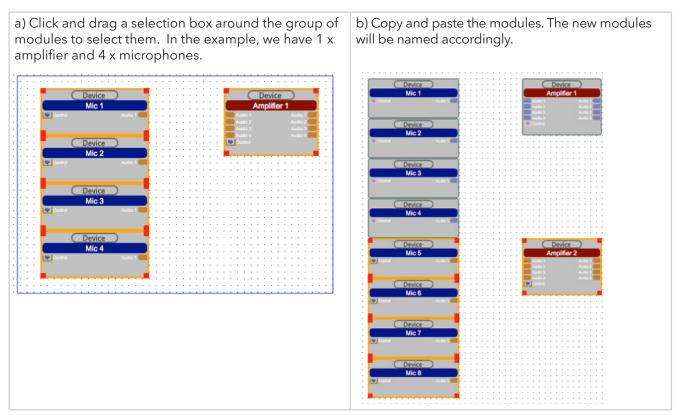
This method works with all design elements and DSP modules in a design.
