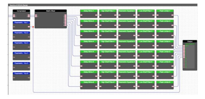
3. Click and drag the corner node to adjust the single wire point. The design schematic may need to be adjusted to make room for the wires.
