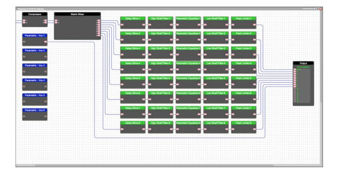
4. Click and drag the corner node to adjust the single wire point. The design schematic may need to be adjusted to make room for the wires.
