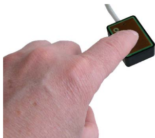
Senso PAD - Capacitive push button
